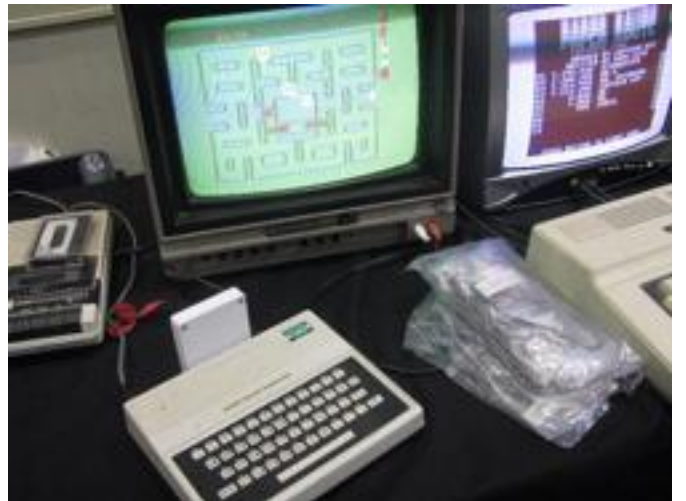
CoCoMan showcased his wares with an MC-10 and a few CoCos, along with his Switch-A-Roo, Walla-V-Cable and Rookaburra Cable, among other items. The Switch-A-Roo is an easy way to connect the CoCo 3's RGB output to a modern-day VGA monitor.
